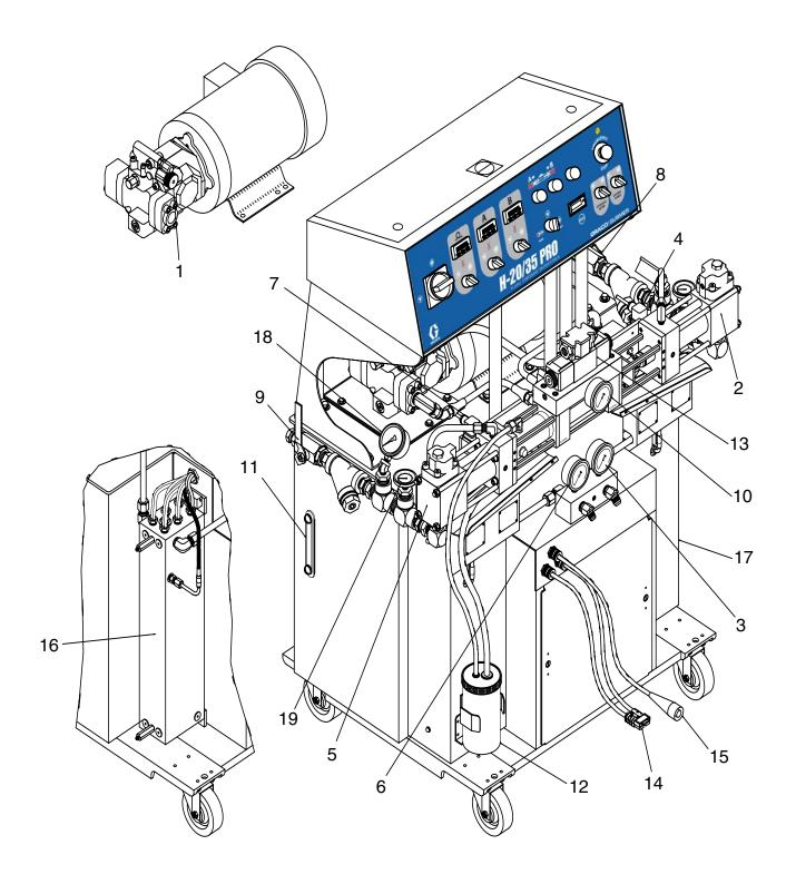
Fig. 2: Component Identification - Main Components
