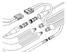
Fig. 12: Hose Connection (step a)
