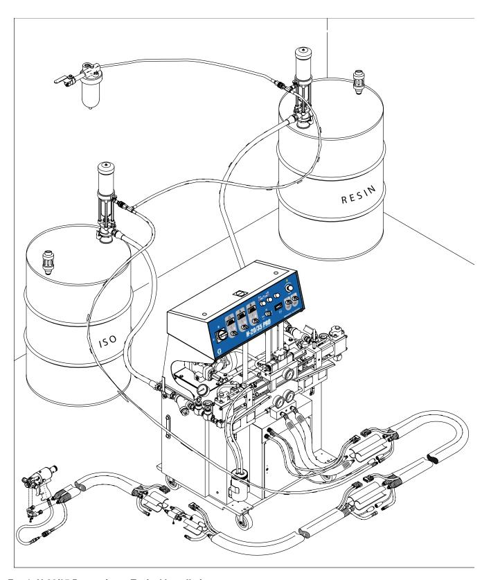
Fig. 1: H-20/35 Proportioner Typical Installation
