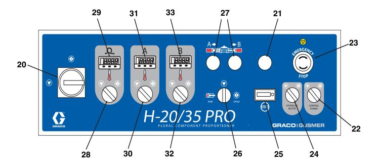
Fig. 4: Component Identification - Front Controls
