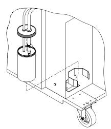
Fig. 10: Lubricant Reservoir Installation
