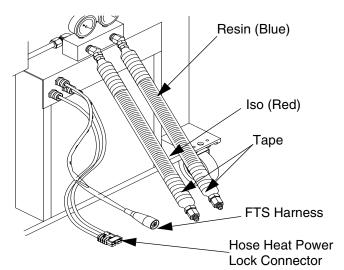
Fig. 11: Isolation Hose Connections
